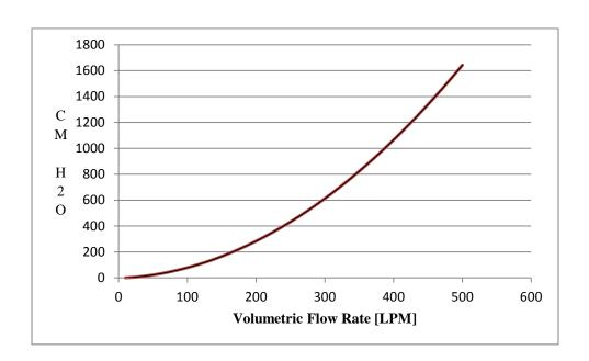
Sensor Pressure Drop Vs. Flow Rate
